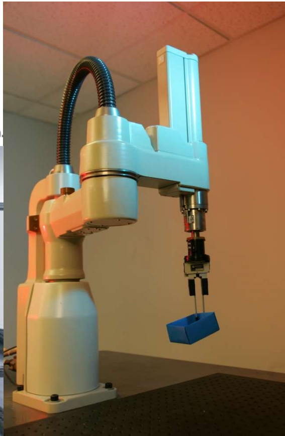
Figure 5. SCARA - Selective Compliance Assembly Robot Arm.
